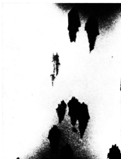
Fig. 4. Nuclei on the (110) face. c-axial vertical ( 100\times ).
